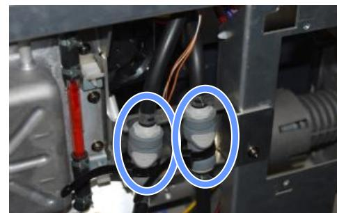
[4] Loose three shafts and remove the 2K PRISM ASSY.
