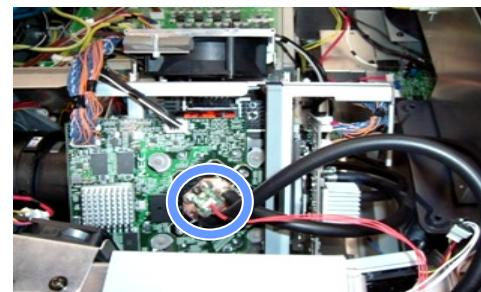
[3] Remove the two liquid cooling tubes.
