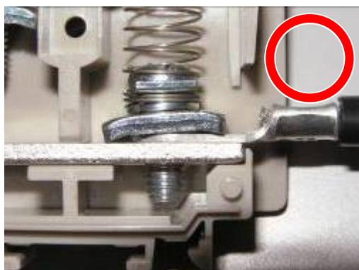
When the cable wire has become pinched due to using a solderless terminal with dimensions other than as designated
