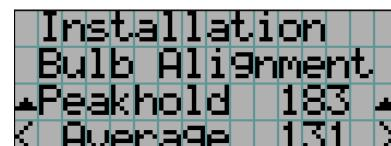
**[4] Adjust the Z-axis adjustment screw to have the maximum bulb alignment.**
