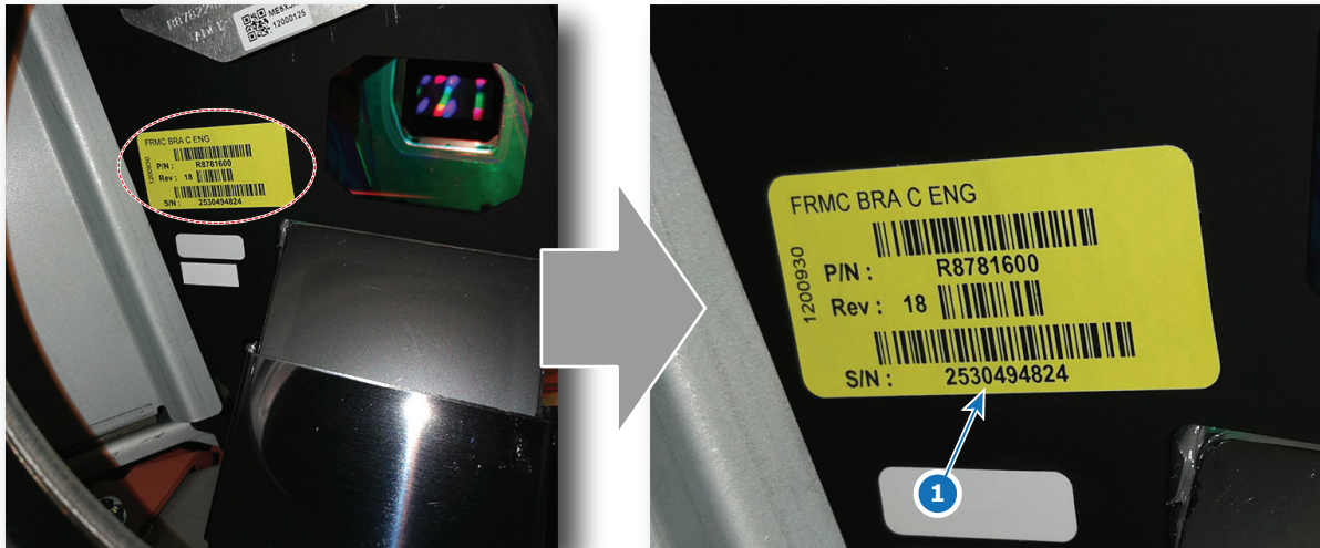
Image 11-1 Location of the label with the serial number of the light processor of an SPxK-series projector.
