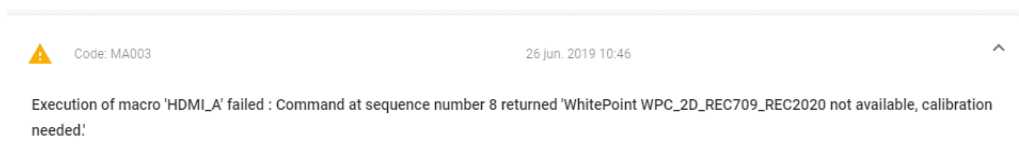
Image 16–29 Example of a failed Macro notification. In this specific example, playing content via HDMI failed because the user forgot to calibrate the projector for the correct color spectrum.
