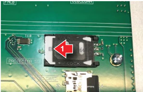
Image 13-15 Removing the projector ID card
