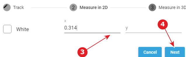
Image 10–5 White Point calibration - 2D measurement
