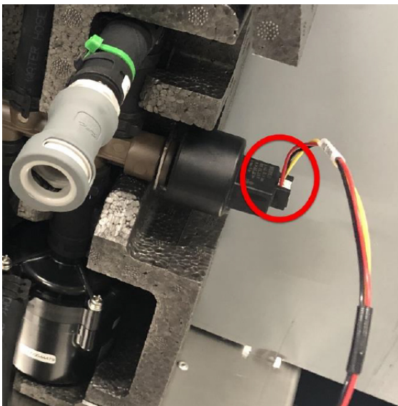
Image 6-31 Location of the pressure sensor on the pump assembly
