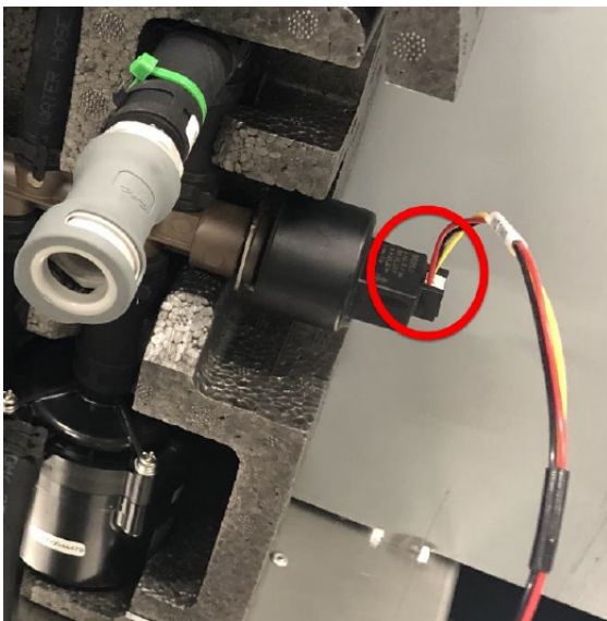
Image 6-26 Location of the pressure sensor on the pump assembly
