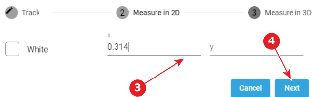
Image 10–5 White Point calibration - 2D measurement
