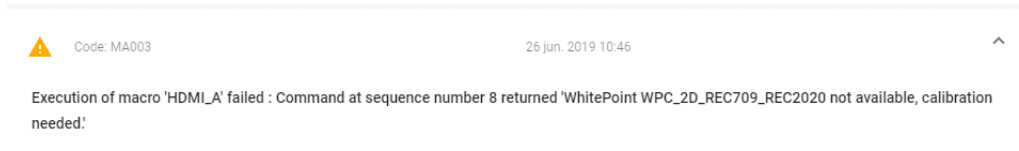
Image 17–41 Example of a failed Macro notification. In this specific example, playing content via HDMI failed because the user forgot to calibrate the projector for the correct color spectrum.
