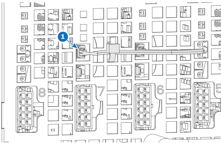
Image 5-28 Example of power board wiring, here between the power modules in slot 6 and 7.
