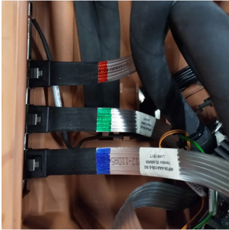
Image 13–53 Location of the three high-speed cables as seen from the front side of the projector
