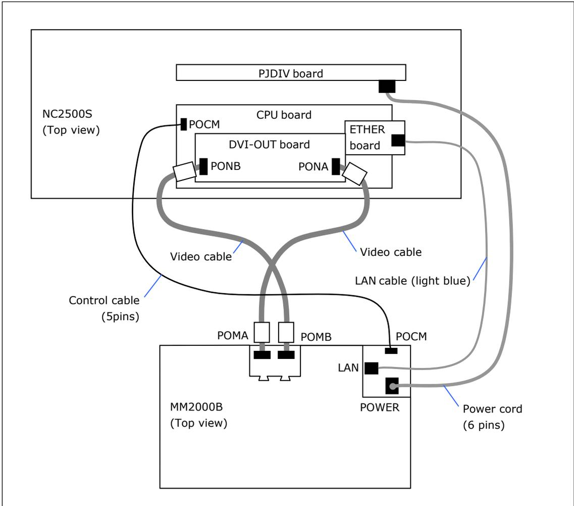
**Note** Both ends of POMA and PONA connector and video cable (either one) are marked in green. Connect the video cables between POMA and PONA and between POMB and PONB. If you connect inappropriate video cable, the video images are not projected.
