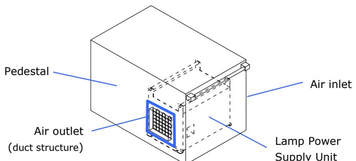
**Example where the lamp power supply unit is installed to the Pedestal (NC-PD01)**
