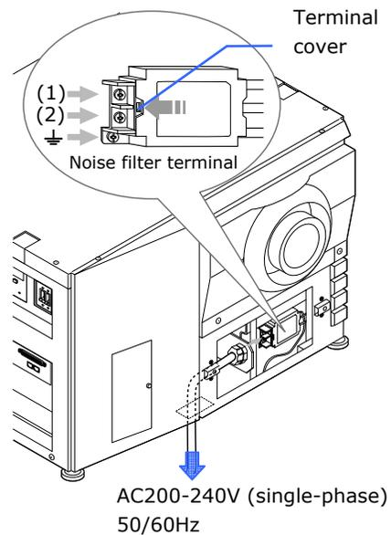
Upon connection completion, close the terminal cover of the noise filter terminal.
