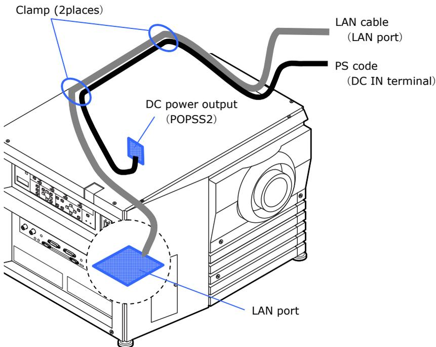
Using the bushing supplied with the holder arm, pass the power cord and LAN cable through the hole in the holder arm to the projector head.
