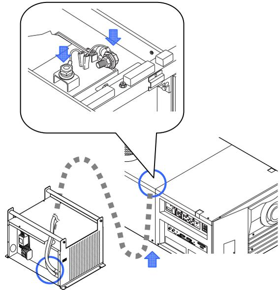
**[8]** Check the setting of the input power selection switch.
