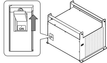
**[3]** Turn the main power switch on the side of your projector head to on.
