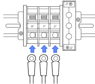
Insert the solderless terminal into the fixing hole of the connecting terminal and tighten the screw with a Phillips-head type screwdriver.
