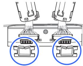
**[3]** Connect the control cable to the NC2500S.
