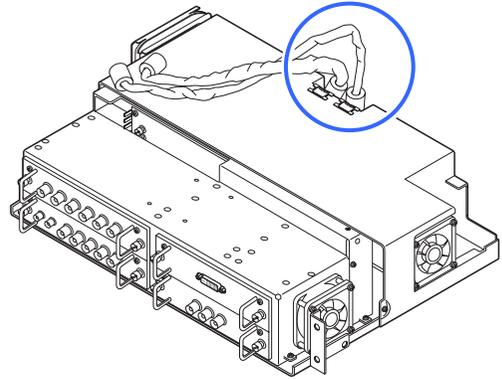
**[2]** Pass the video cables respectively to the clamps of MM2000B.
