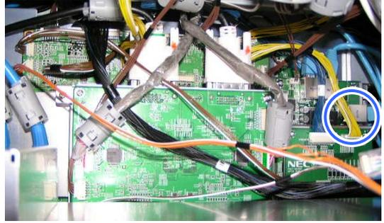
**[6]** Temporarily mount MM2000B (insert it for about 1/3) to the NC2500S.
