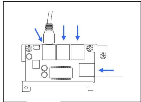
**[7]** Bundle an extra length of the cable to the PC board.
