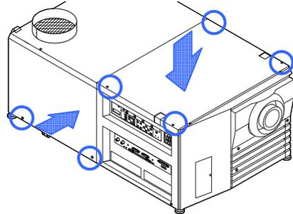
This completes the connection of the power cord. Next, mount a primary lens (Keep the front cover (bottom) of the projector removed here).
