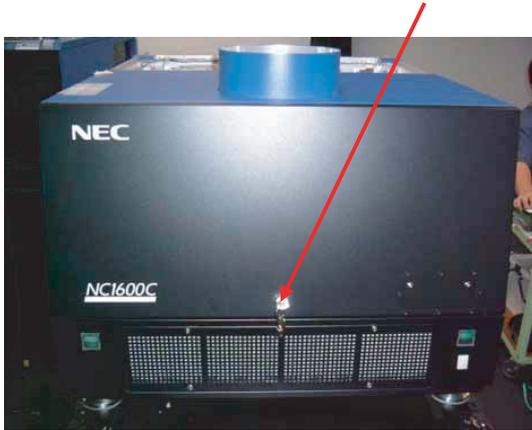
3. Loosen four screws of the lamp cover and remove the cover.
