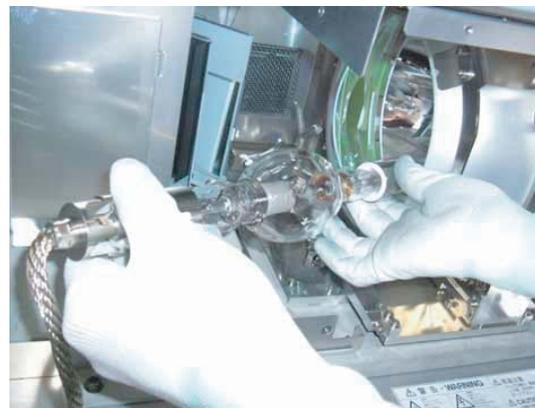
Never touch the glass parts of the lamp bulb and the reflector mirror surface. In case of touching them, wipe the parts as per Caution 1.
