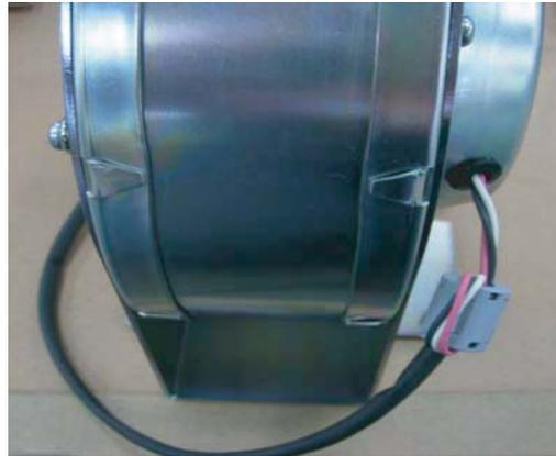
② Set Fan after attaching Cushion and Collar on DC Fan BL6771.
