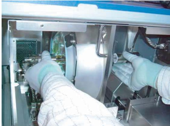
Remove the bulb from the reflector.
