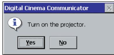
The projector is turned on and starts the starting process. The progress bar is displayed during the starting process (for about 40 sec.).
