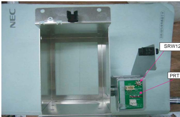
② Attach TAMPER PWB on BRACKET (TAMPER) A.
