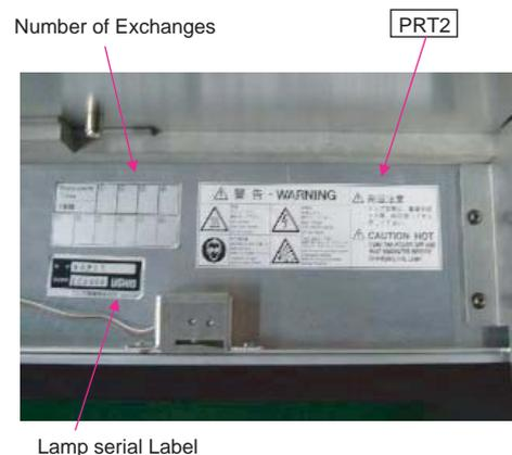
**Confirm that installation of the Lamp Cover S Assy has been completed. Subsequent work can be carried out outside the exclusive lamp mounting room.**
