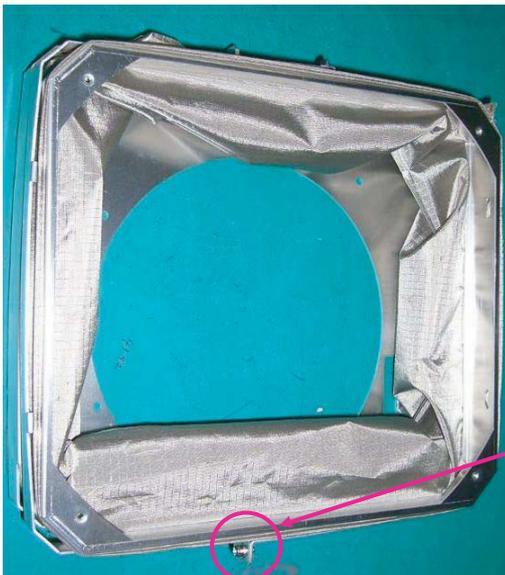
Caution : When fastening the Holder (Shield) A and the Holder (Shield) B with screws, confirm that the screws are not located on the Connector side of the Lens Mount (PA67), but on the opposite side (lower side).
