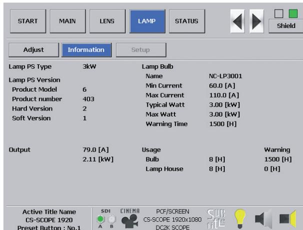
**NOTE** If the projector head is being used with the NC800 series, the Lamp information display (The [Information] button) is unavailable.
