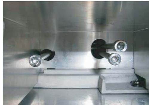
**After the fixing band has been cut, handle the Reflector Base (PA67) carefully so that the Lamp Bulb block and the Reflector block are not damaged by the wires of the anode and cathode blocks as a result of coming in collision with them.**
