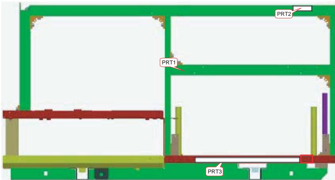
PRT2 should be pasted on beside the Bracket T attachment.
