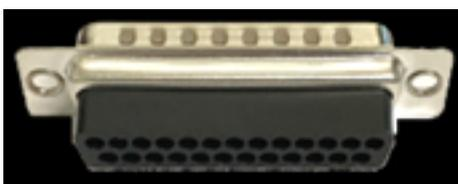
*Figure 108: 25-pin D-connector back*
