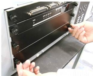
6. Slide the Dolby IMS3000 board into the projector media block slot.
