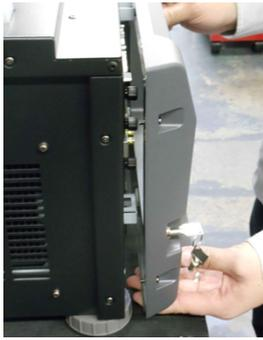
9. Tighten the four screws.
