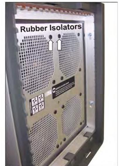
**Figure 5-16 Remove Light Engine Fan Pack**
