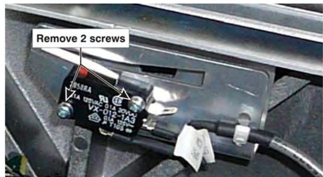
**Figure 5-56 High Security Interlock**
