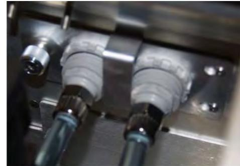
**Figure 5-33 Liquid Cooling Quick Disconnects**
