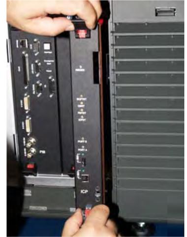
**Figure 5-28 Remove ICP**
