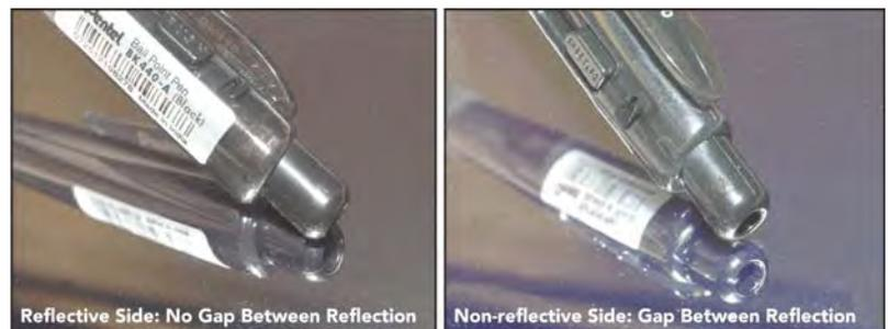
**Figure 5-20 Reflective vs. Non-Reflective Surfaces**
