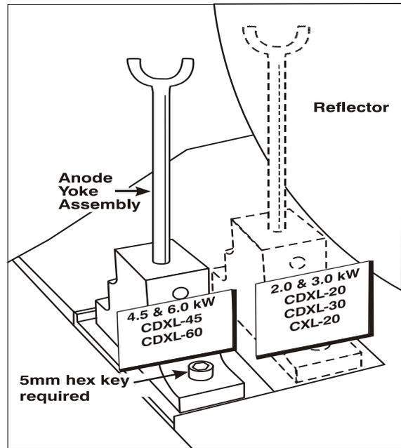
Figure 2-21 Yoke assembly installation
