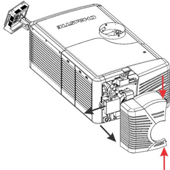
Figure 2-12 Shroud Removal
