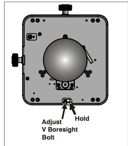
Figure 4-6 Adjust Vertical Bore-sight Bolt
