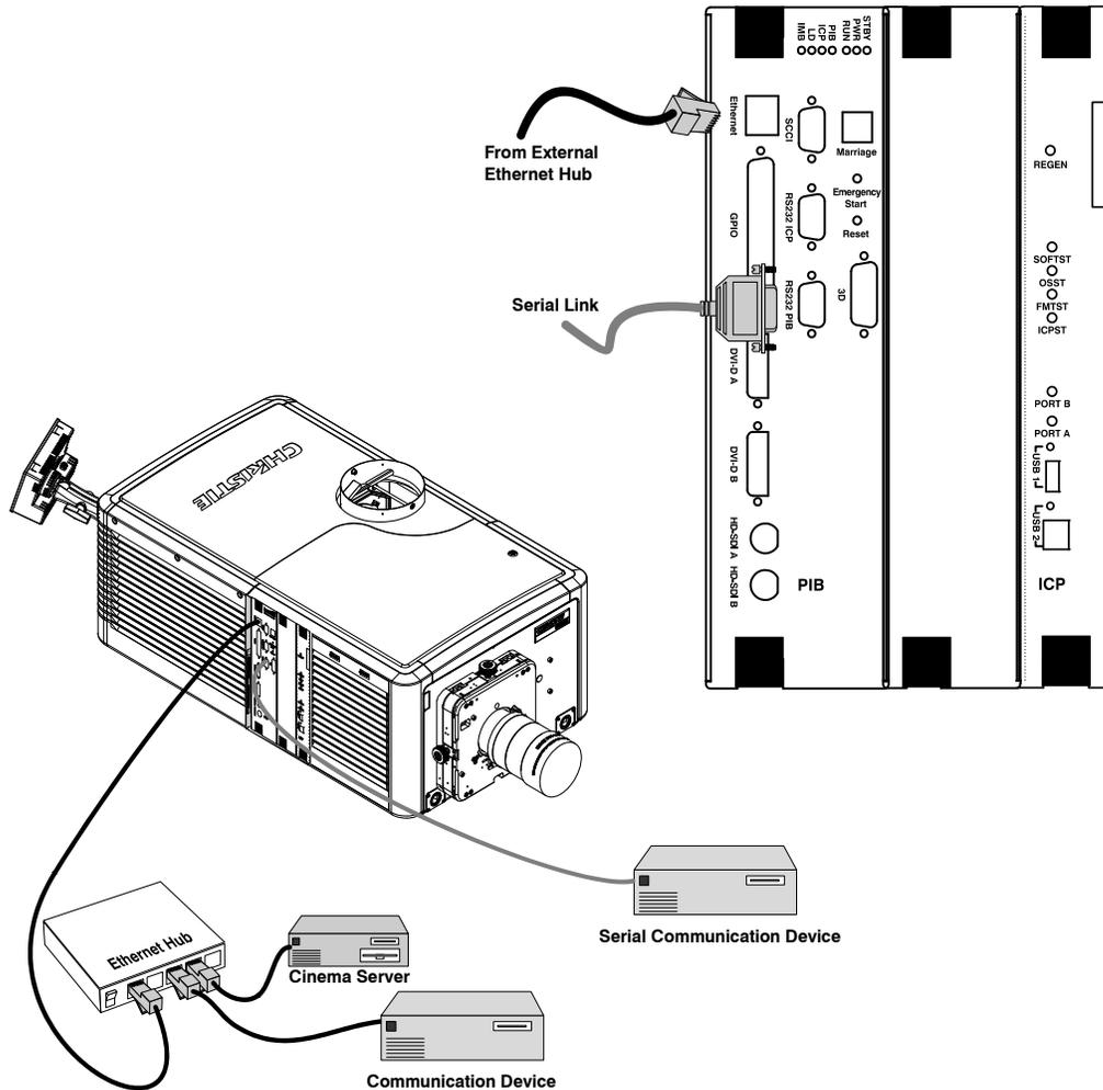
**Figure 3-1 Connecting Communications**
