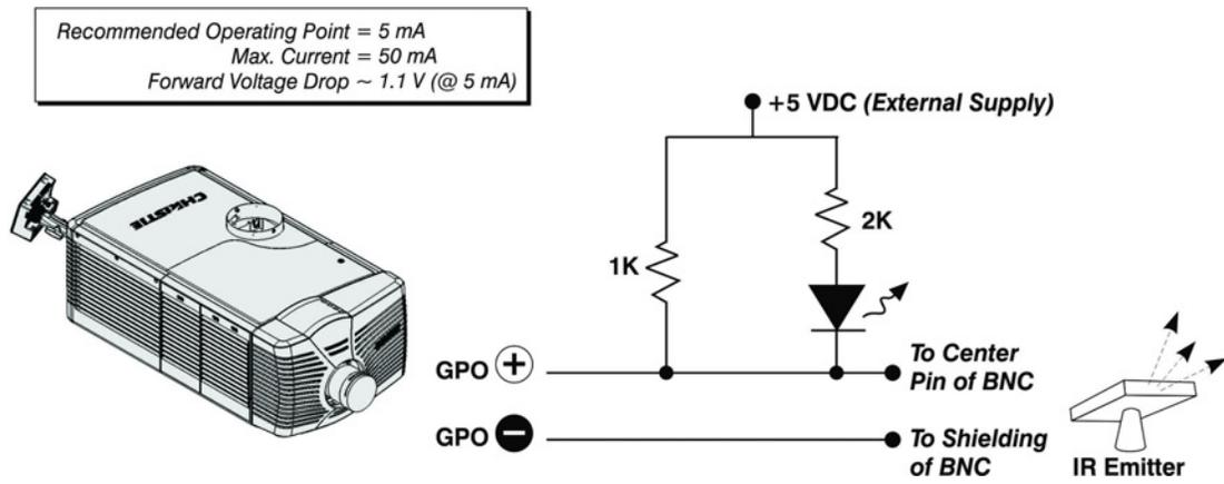
**Figure 3-3 GPIO Circuit Diagram**
