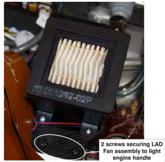
Figure 5-15 Remove LAD Fan Assembly
