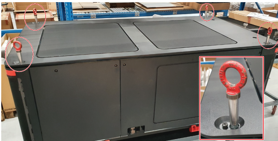
Image 2-5 Example of eye bolts mounted in the top cover
