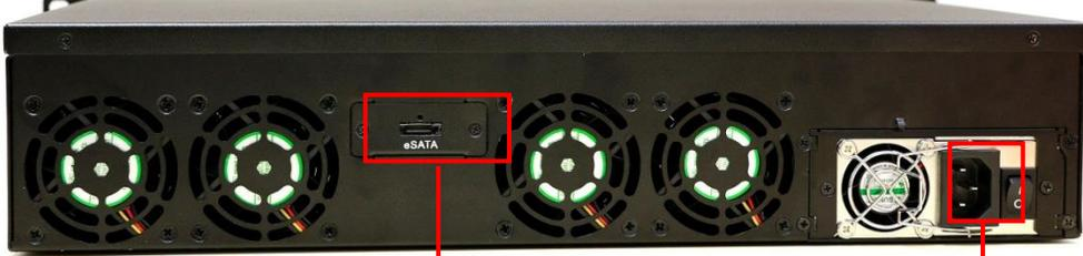
The image shows the back panel of the Enterprise Storage unit. It features four green-lit fans on the left and a power connector on the right. A red box labeled '2' highlights the eSATA connector, and another red box labeled '1' highlights the power connector.
