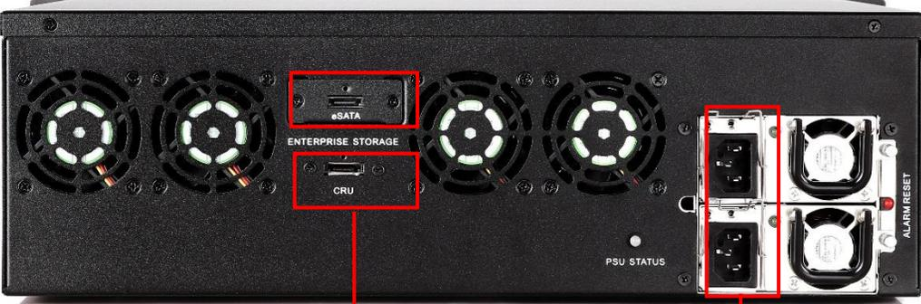
The image shows the back panel of the Enterprise Storage Plus unit. It features four green-lit fans on the left and two power connectors on the right. A red box labeled '3' highlights the CRU connector, another red box labeled '2' highlights the eSATA connector, and a third red box labeled '1' highlights the power connectors.
