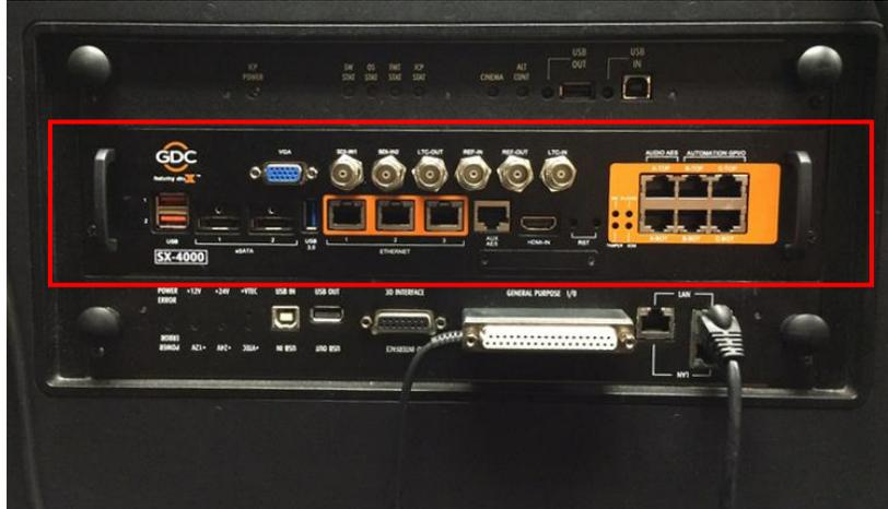
Figure 7 Inserting SX-4000 into the projector.
