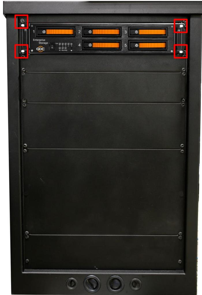
Figure 10 Put the Enterprise Storage on pedestal.
