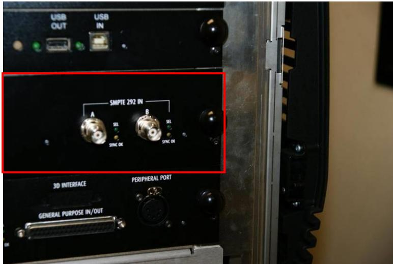
Figure 3 Remove interface board from Barco projector.
