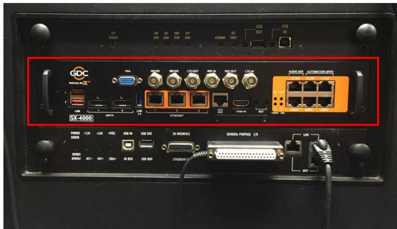
Figure 4 SX-4000 Placement on Barco projector.
