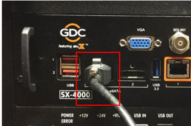
Figure 13 Insert the eSATA cable into SX-4000 eSATA port 1.
