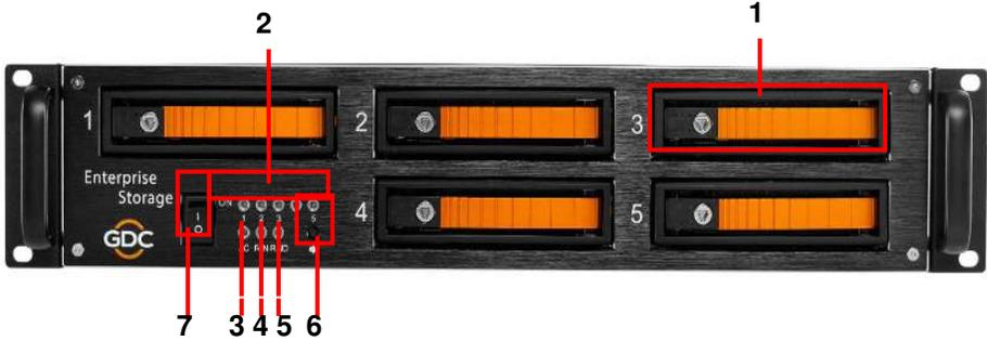
The image shows the front panel of the Enterprise Storage device. It features five HDD trays labeled 1 through 5. Callout 1 points to the HDD Tray in tray 3. Callout 2 points to the HDD LED in tray 2. Callout 3 points to the Power LED. Callout 4 points to the Fan LED. Callout 5 points to the RAID LED. Callout 6 points to the Buzzer Mute Button. Callout 7 points to the Power Switch.
