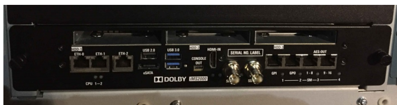
Figure 4-8 IMS2000 Inserted Without Hard-Disk Drives
