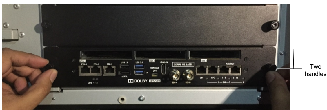
Figure 4-9 Securing the Board
