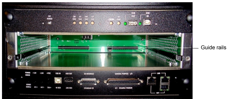
Figure 5-3 Empty Media Block Slot
