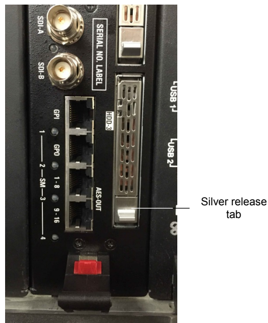
Figure 6-6 Silver Latch on Hard-Disk Drive
