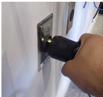
Figure 6-14 Connecting the Power Cable
