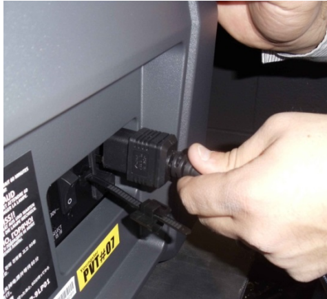
Figure 4-21 Connecting the Power Cable
