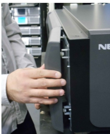
Figure 4-15 Reattaching the Filter Cover
