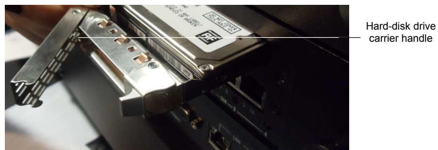
Figure 5-6 Inserting Hard-Disk Drive
