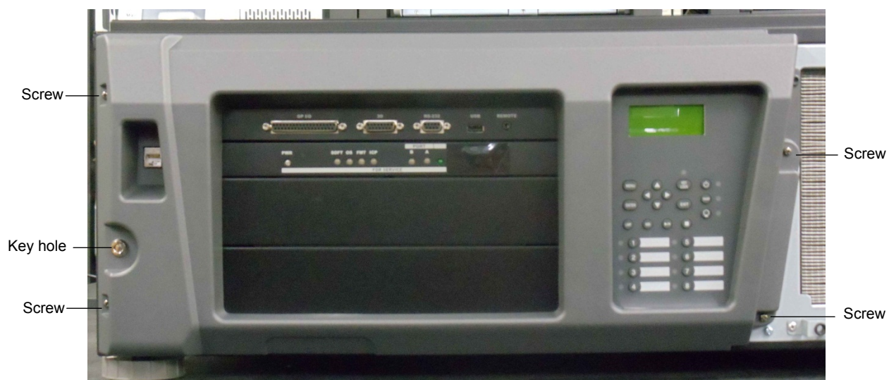
Figure 4-3 Removing Filter Screws
