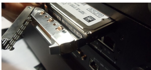
Figure 15-1 Hard-Disk Drive Removal
