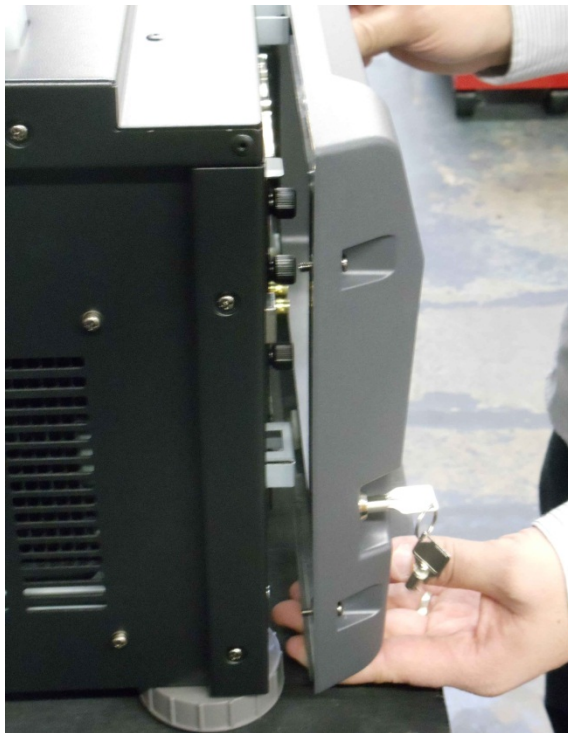
Figure 4-13 Reattaching the Projector Cover
