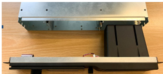
Figure 5-16 Remove Front Panel from the Chassis
