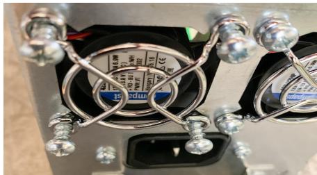
Figure 5-10 Remove Screws From Fans
