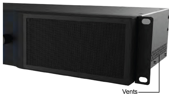
Figure 2-2 Ventilation Cutout Locations
