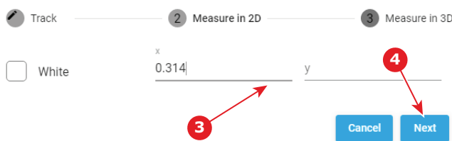
Image 9–5 White Point calibration - 2D measurement
