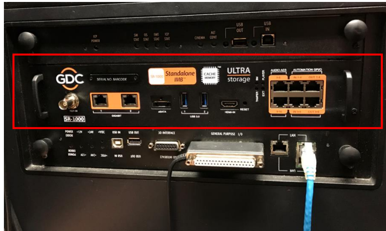
Figure 7: Installing the SR-1000 into the projector
