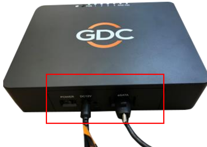
Figure 8: Connect eSATA cable to the Portable Storage
