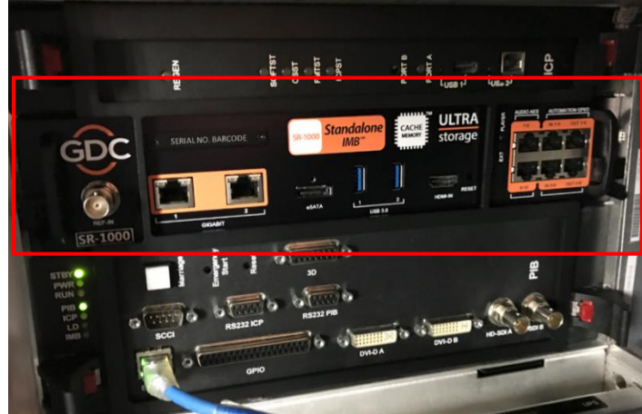
Figure 5: SR-1000 Placement on Christie projector
