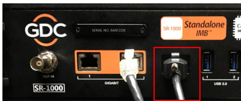
Figure 9: Insert eSATA cable into SR-1000 eSATA port
