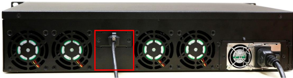
Figure 10: Connect eSATA cable to the Enterprise Storage
