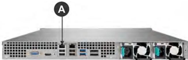
3. Connect the other end of the Ethernet cable to the secondary Ethernet port of a second Christie NAS.
