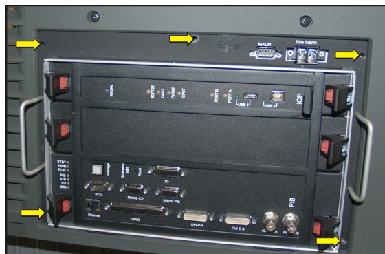
Figure 5-53 Remove Screws Securing Cardcage
