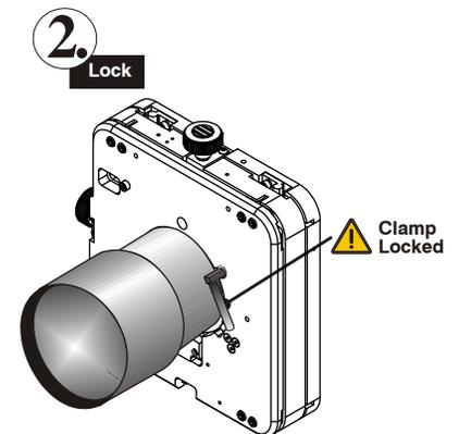
**Figure 2-9 Lock Lens In Place**
