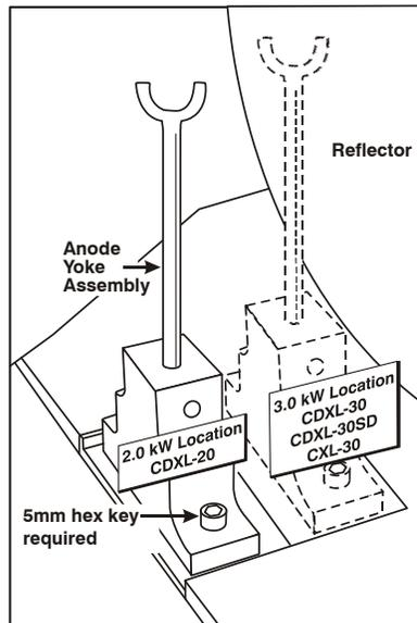
**Figure 2-10 Anode Yoke Posi-**
