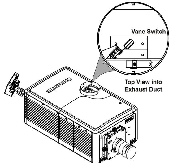
Figure 2-7 Exhaust Duct Vane Switch
