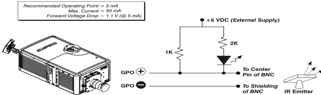
**Figure 3-4 GPI Circuit Diagram**
