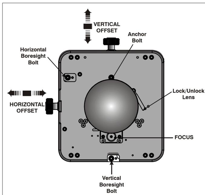
**Figure 4-1 Standard Lens Mount**
