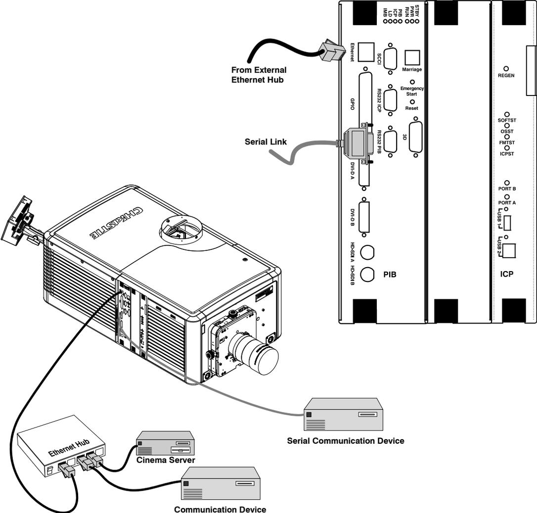
**Figure 3-2 Connecting Communications**
