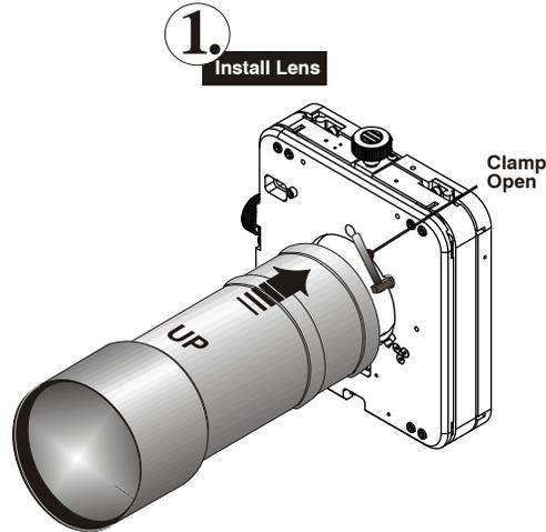
**Figure 2-8 Open Lens Clamp and Insert Lens**
