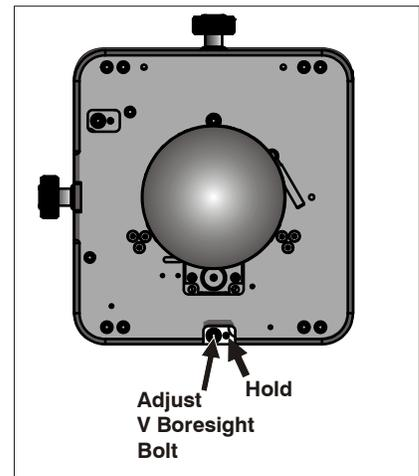
**Figure 4-6 Adjust Vertical Bore-sight Bolt**
