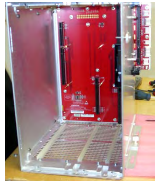
Figure 5-27 Cardcage with Backplane
