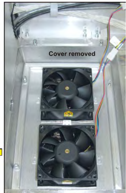
Figure 5-18 Cardcage Exhaust Fans
