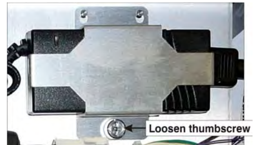
Figure 5-37 Standby Power Supply
