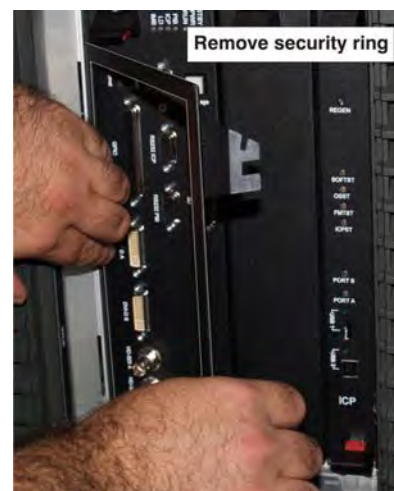
Figure 5-25 Remove Security Ring
