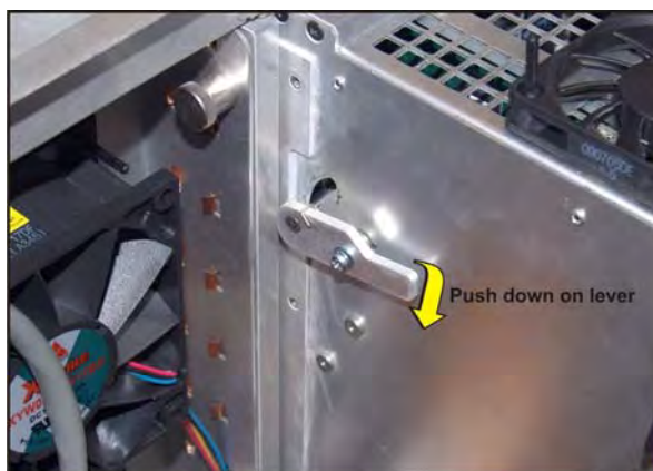
Figure 5-24 Spring Latch for Security Ring
