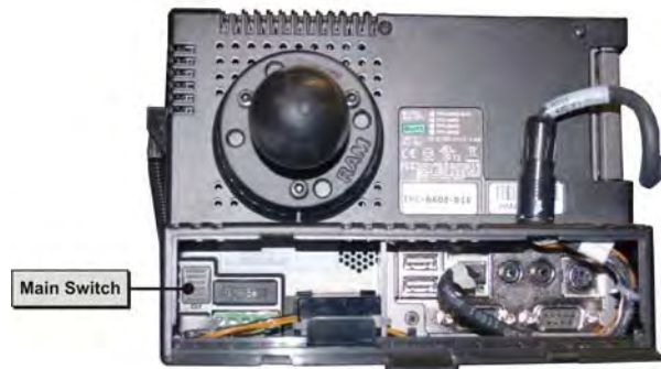
Figure 5-4 Main Switch on TPC-660E
