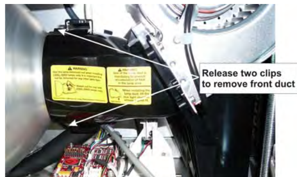
Figure 5-44 Front Lamp Duct
