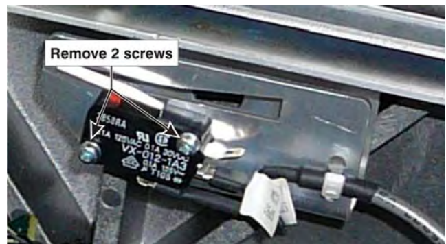
Figure 5-56 High Security Interlock
