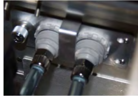
Figure 5-33 Liquid Cooling Quick Disconnects
