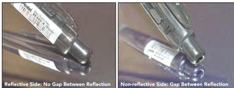
Figure 5-20 Reflective vs. Non-Reflective Surfaces
