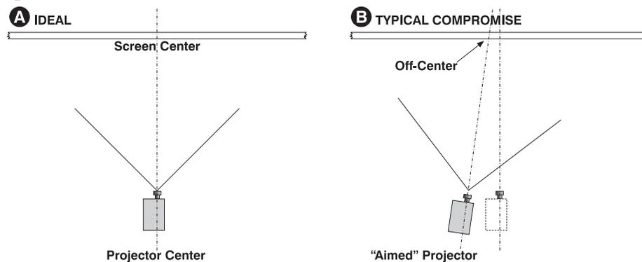
**NOTE:** Keep the cinema projector lens as parallel to the screen as possible, even if significantly above the screen center. When a particularly short throw distance combines with a very wide screen, you may have to forfeit some aim and stay more parallel to the screen. In such cases, some lens offset can reduce the keystone distortion.
