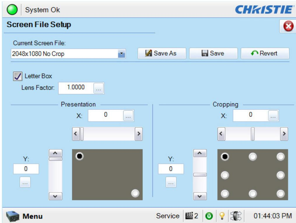
**Figure 6-24 Advanced Setup: Screen File Setup Window**
