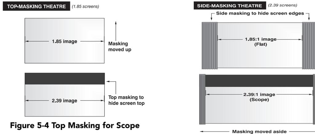
Figure 5-4 Top Masking for Scope
