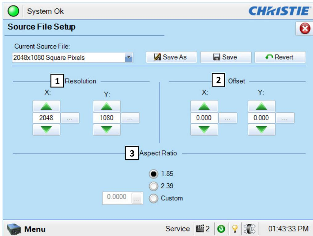
**Figure 6-23 Advanced Setup: Source File Setup Window**
