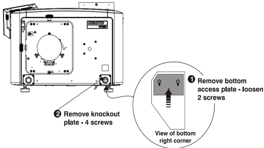
2. Remove the knockout plate located in the bottom right corner of the front bezel. The AC supply is routed to the terminal block through a strain relief mounted on this knockout plate.
