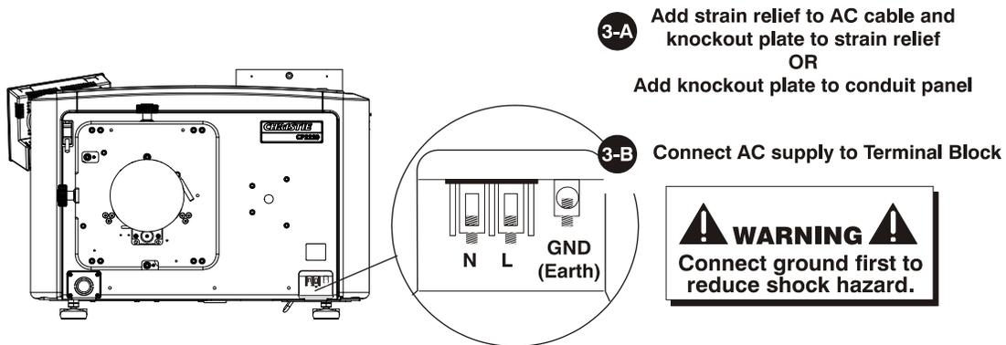
4. Replace the knockout plate and the bottom access panel over the terminal block.
