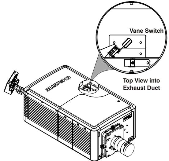
**⚠ CAUTION** Never disable the vane switch. Attempting to operate the cinema projector with inadequate airflow can result in dangerous overheating of the cinema projector.
