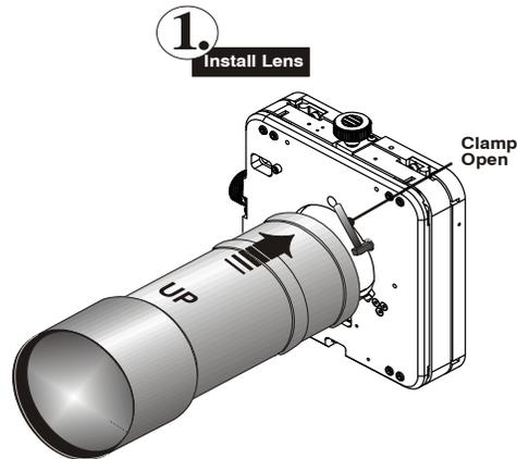
3. With the UP label facing up, insert the lens straight into the lens mount opening all the way back, without turning.
