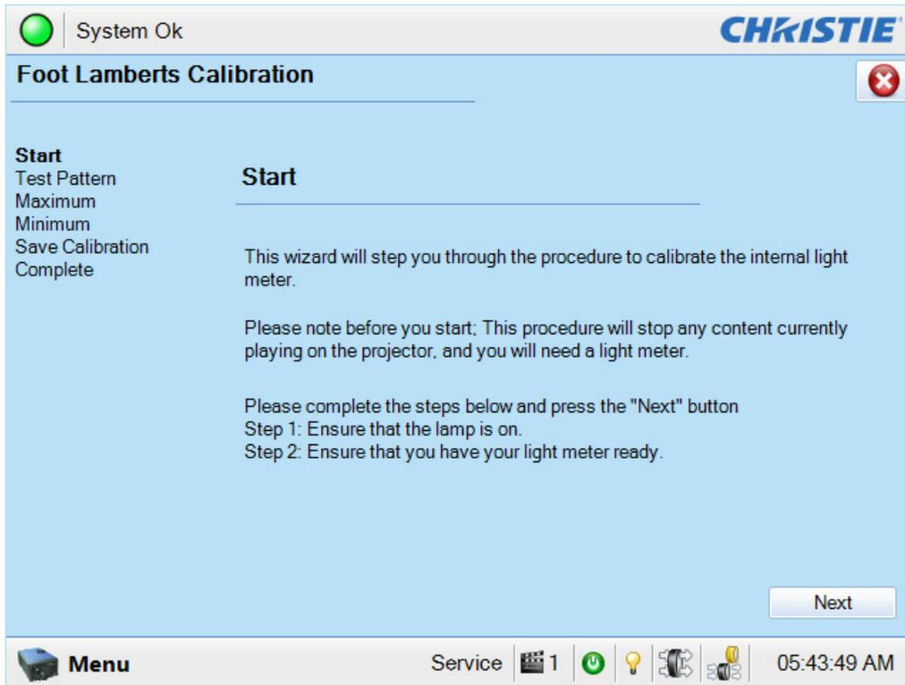
Figure 6-38 Administrator Setup: Foot Lamberts Calibration Start Window
