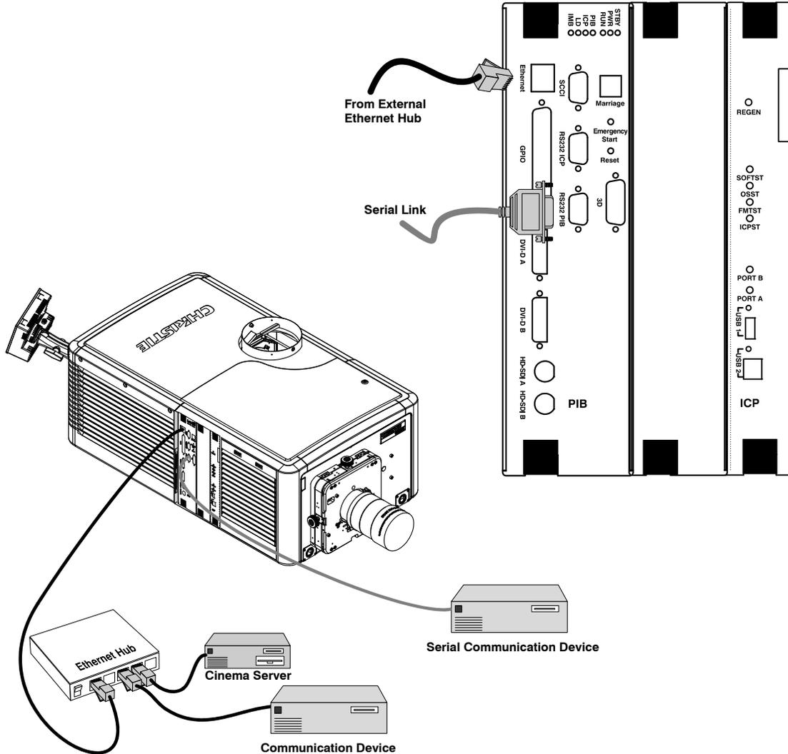
Figure 3-2 Connecting Communications
