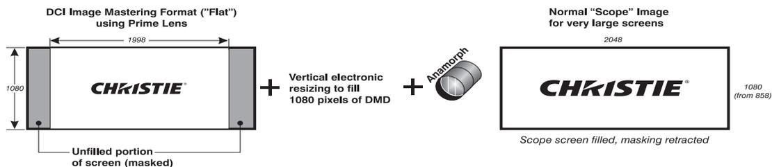
Figure 5-2 Using Anamorphic Lens to Achieve "Scope" for Large Screens
