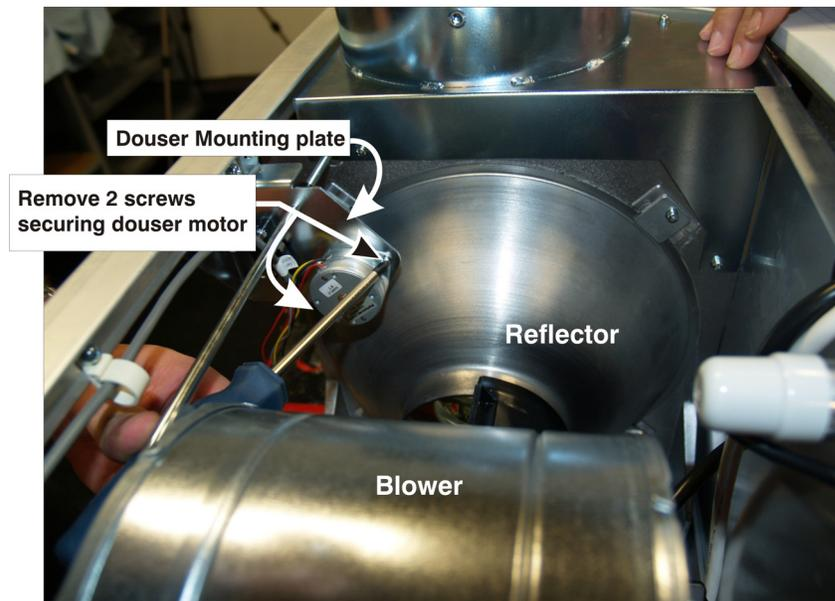
FIGURE 1-18 REMOVE DOUSER MOTOR
