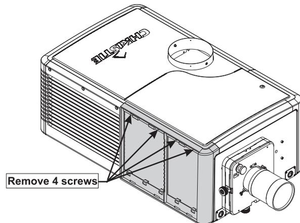
**FIGURE 1-7 REMOVE ACCESS PANEL FRAME**
