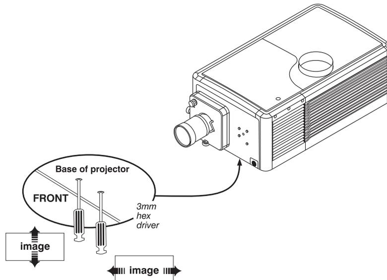
FIGURE 1-28 ADJUST FOLD MIRROR
