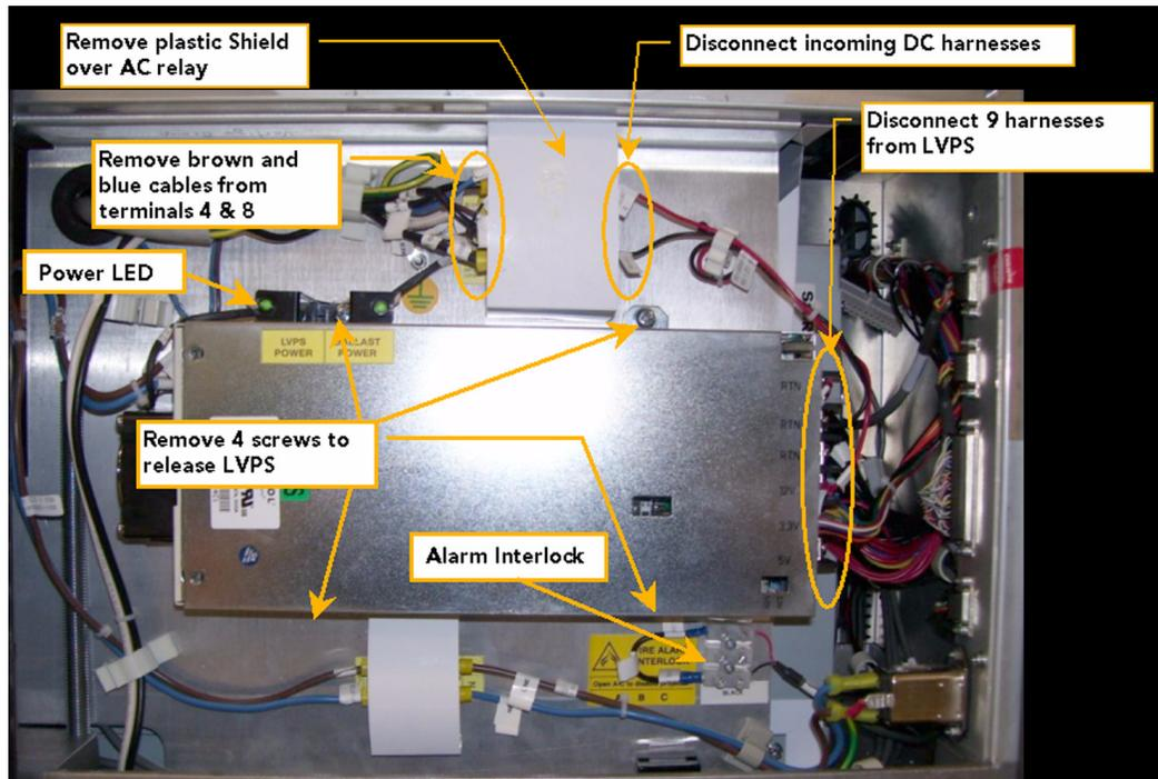
**FIGURE 1-51 REMOVE LOW VOLTAGE POWER SUPPLY**
