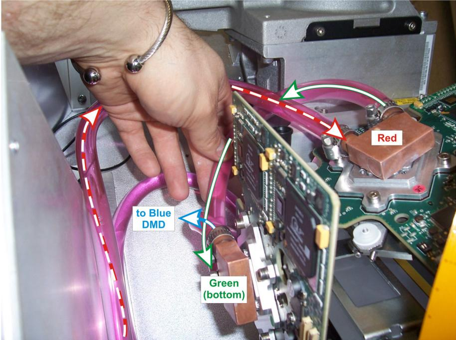
FIGURE 1-47 COOLANT HOSE ROUTING FROM HEAT EXCHANGER TO RED DMD
