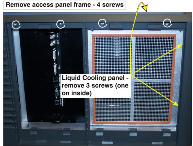
**FIGURE 1-22 REMOVE LIQUID PANEL SCREWS**
