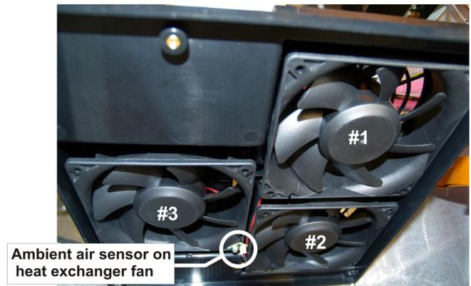
Intake fans - view from the back of the mounting panel
