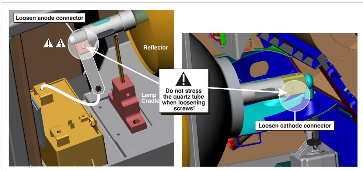
**FIGURE 1-33 LOOSEN CATHODE (-) AND ANODE (+) CONNECTORS TO REMOVE BULB**
