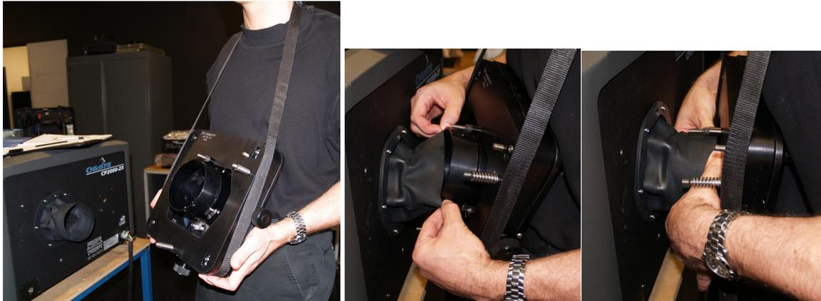
FIGURE 1-40 INSTALLING THE LENS MOUNT USING THE SUPPLIED STRAP
