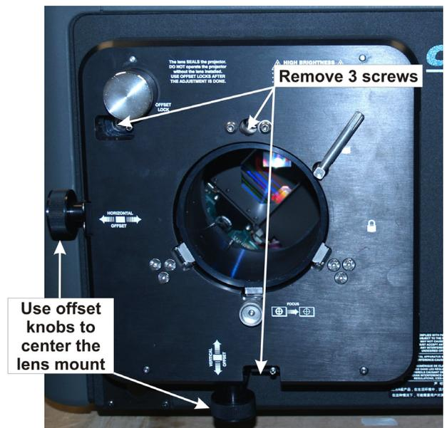
**FIGURE 1-39 LENS MOUNT REMOVAL**
