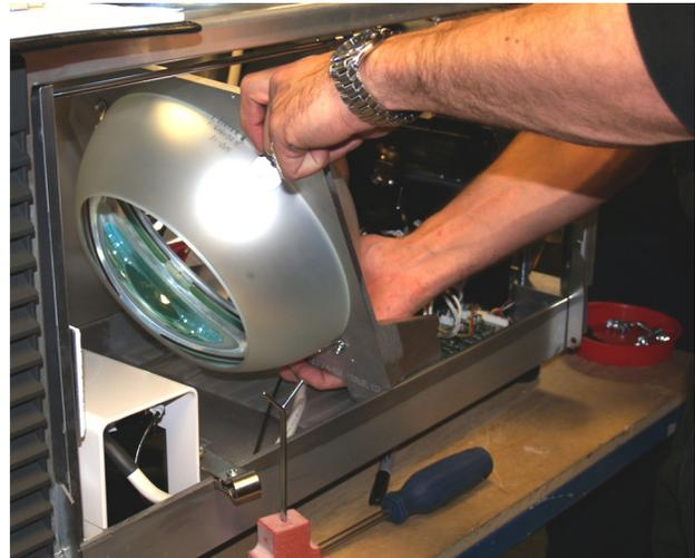
**FIGURE 1-55 REMOVE REFLECTOR**
