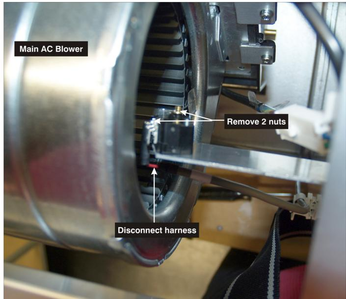
FIGURE 1-62 MAIN BLOWER VANE SWITCH
