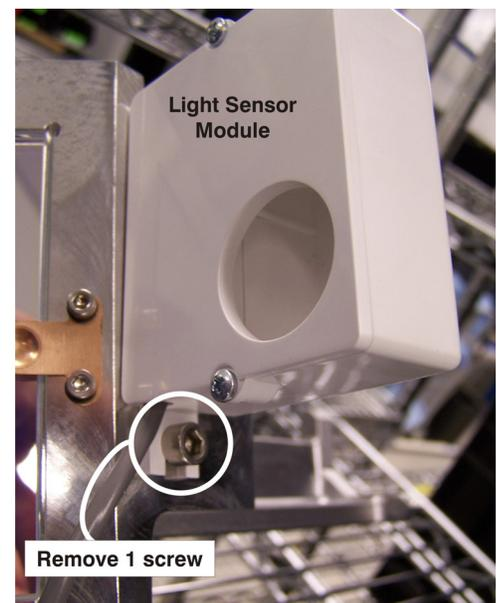
**FIGURE 1-42 REMOVE LIGHT SENSOR MODULE**
