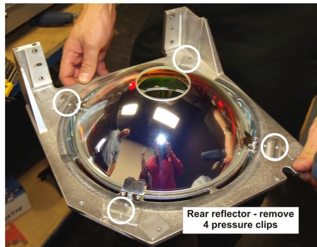
**FIGURE 1-57 REMOVE REAR REFLECTOR**
