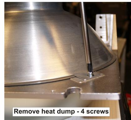
**FIGURE 1-56 REMOVE HEAT DUMP**
