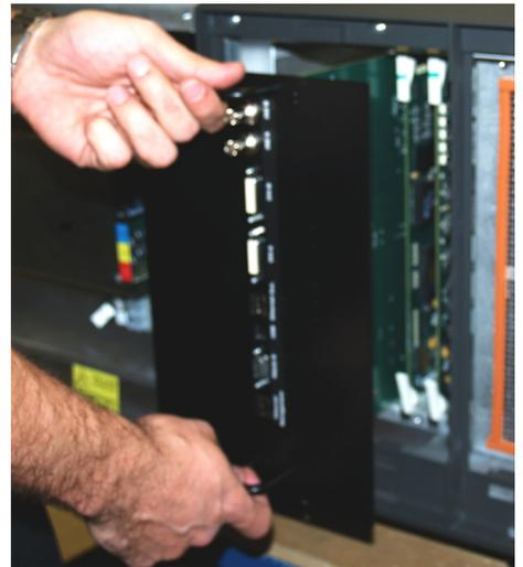
**FIGURE 1-54 REMOVE PCM ASSEMBLY**
