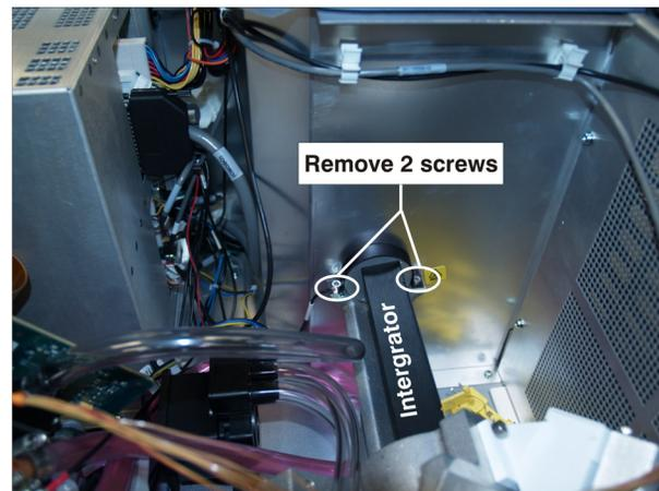
**FIGURE 1-31 REMOVE INTEGRATOR ASSEMBLY**
