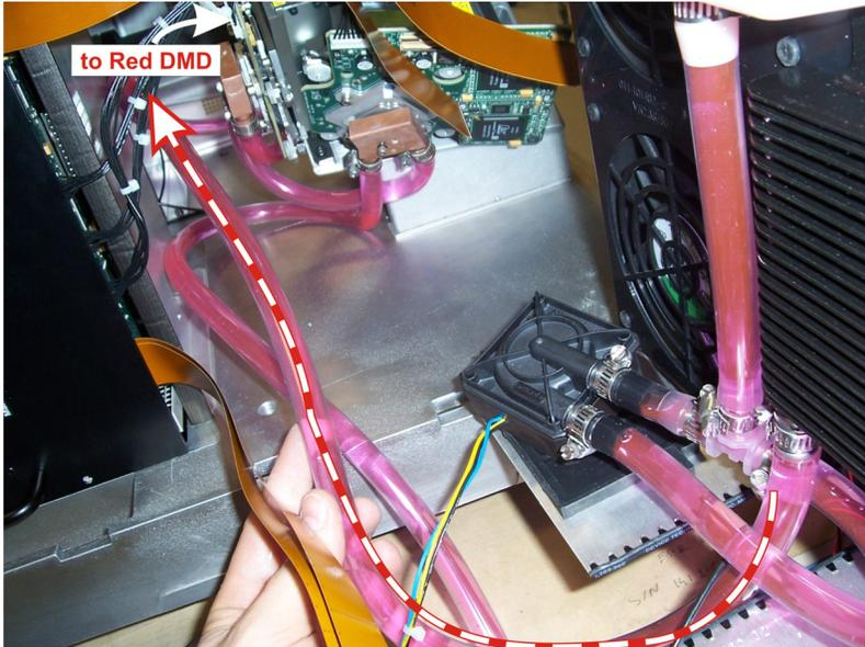
FIGURE 1-46 COOLANT HOSE ROUTING FROM HEAT EXCHANGER
