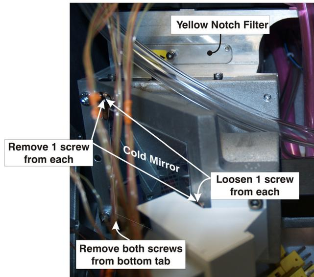
FIGURE 1-15 REMOVE COLD MIRROR
